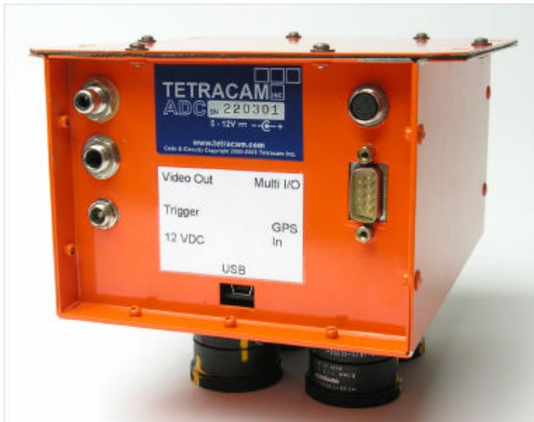
The minimum number of interconnections is two, power and either trigger, USB or the Multi I/O cable. Connection of a video monitor is strongly suggested, it functions as an accurate viewfinder and serves to show the operating state of the camera.
