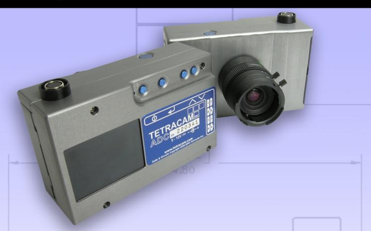
This third generation ADC stands on the shoulders of the venerable 1.3 megapixel camera in use worldwide. It offers higher ground resolution and improved spectral accuracy along with greater flexibility of operation and control. Red, Green and NIR bands (approximating TM2, TM3 and TM4) provide the information needed for extraction of NDVI, SAVI, canopy segmentation and NIR / Green ratios. Standard GPS data capture from an external receiver adds position data to your images.
